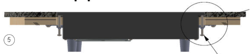
Use the leveling screws to adjust the range height so that it rests flush with countertop
